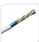
Matassa cavo rete UTP CAT5E 4X2X24AWG, 4coppie x 0.52mm Solid COPPER , OD:5.2 ± 0,2mm PV. KIONIX CAT5 INDOOR UTP 24AWG/4P ISO/IEC11801 EIA/TIA568 CE CPR Eca 001M ~
